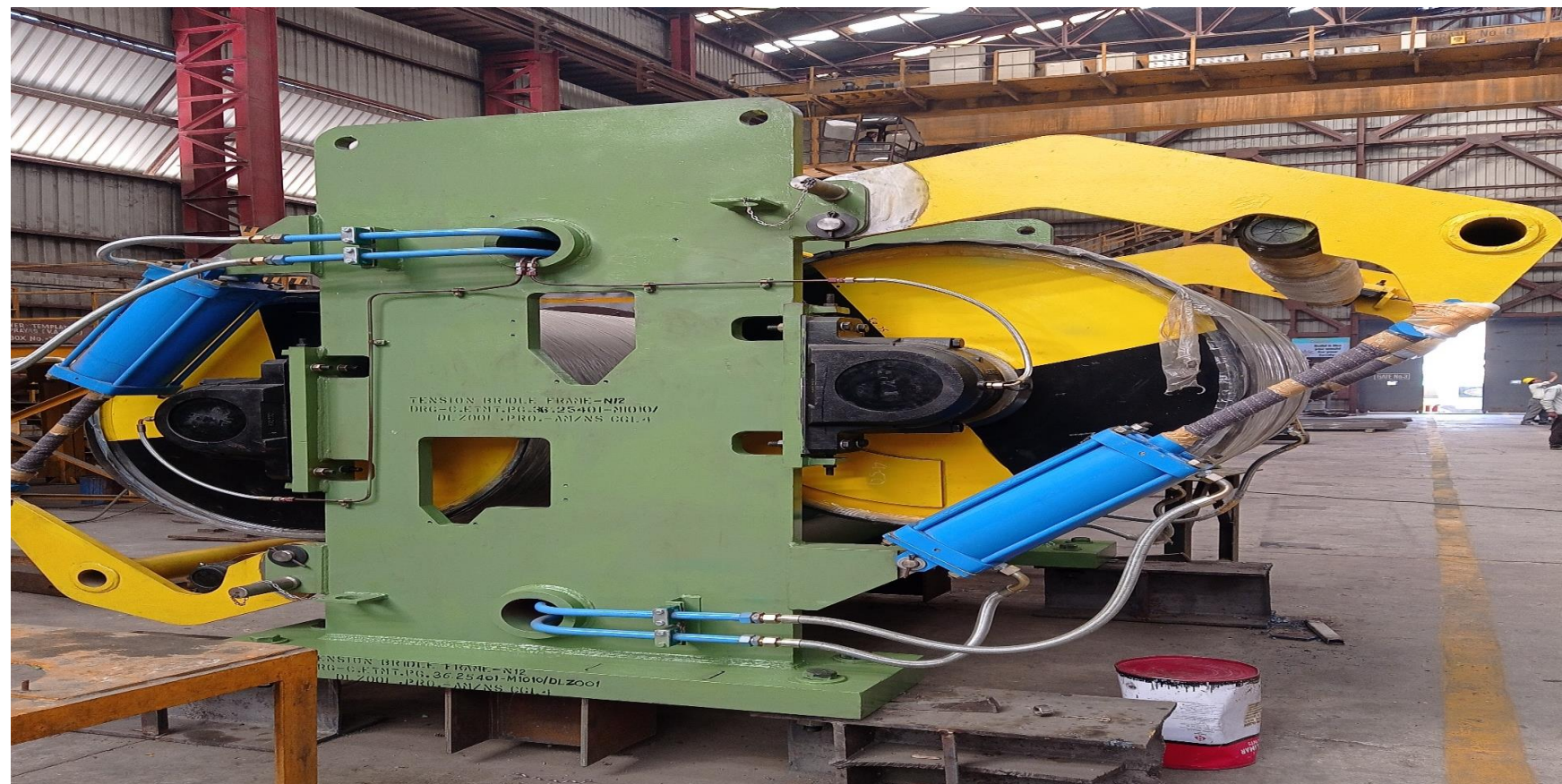
Tension Bridles Galvanization/ Pickling line
