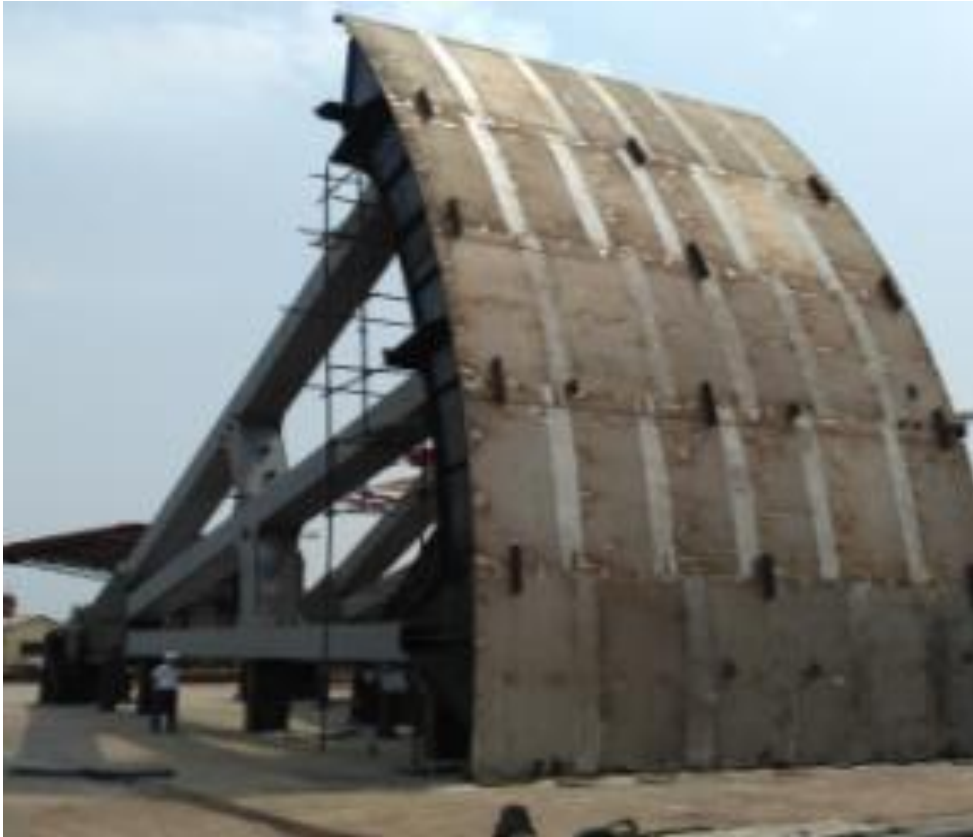
Main Spill Way Radial Gate (Weight 205 Metric Tonne) (8 x 18 x 20) Mts With Arms & Trunion Control Assembly for BHUTAN Hydro Electric Project
