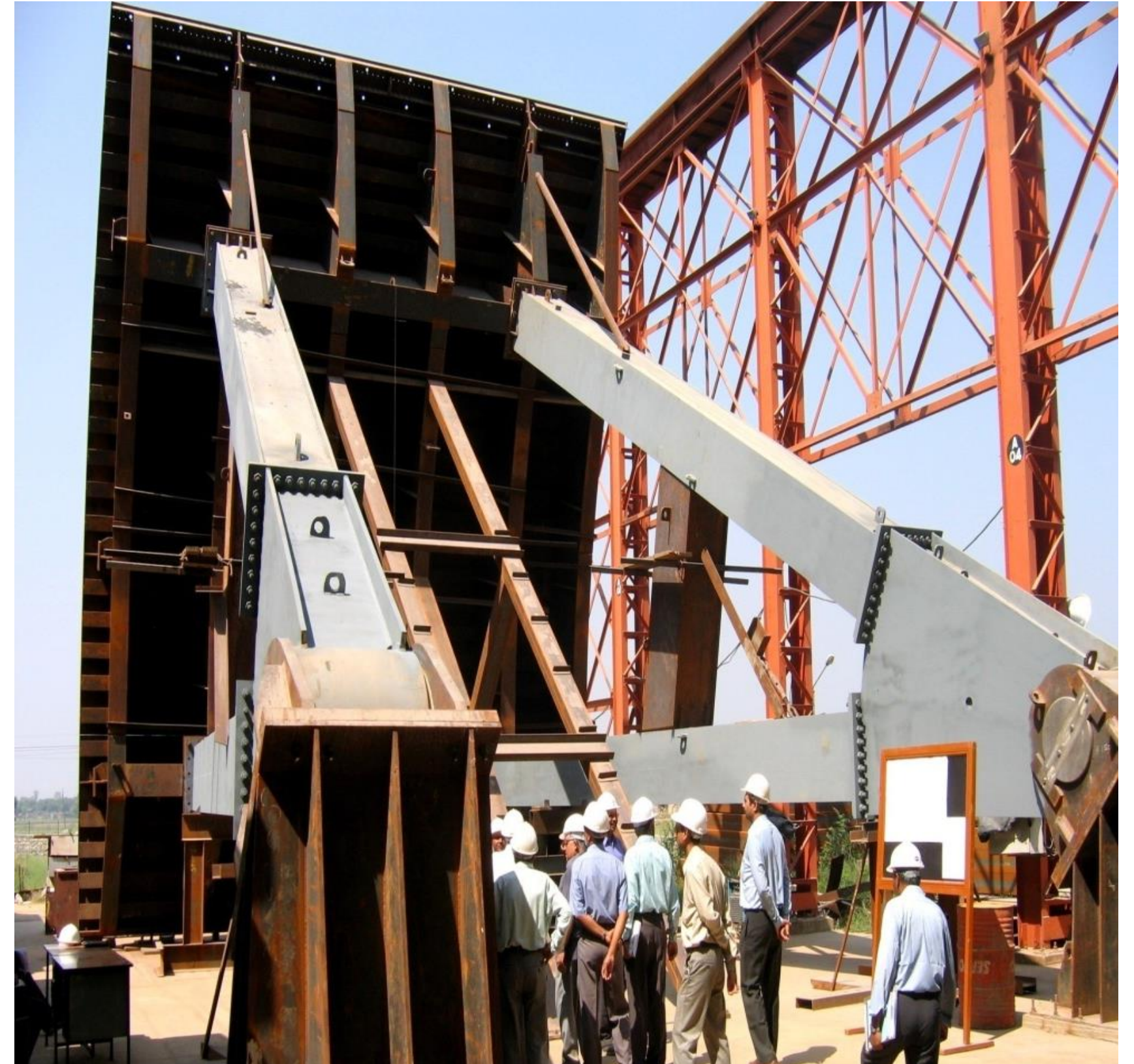
Main Spill Way Radial Gate (Weight 205 Metric Tonne) (8 x 18 x 20) Mts With Arms & Trunion Control Assembly for BHUTAN Hydro Electric Project
