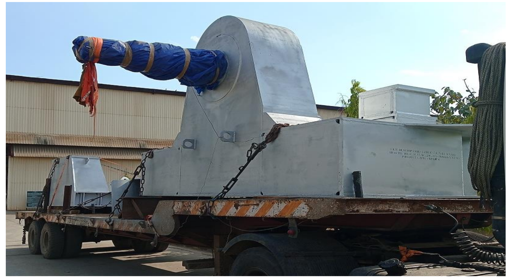
LADLE TILTER (CAPACITY - 350 MT)
