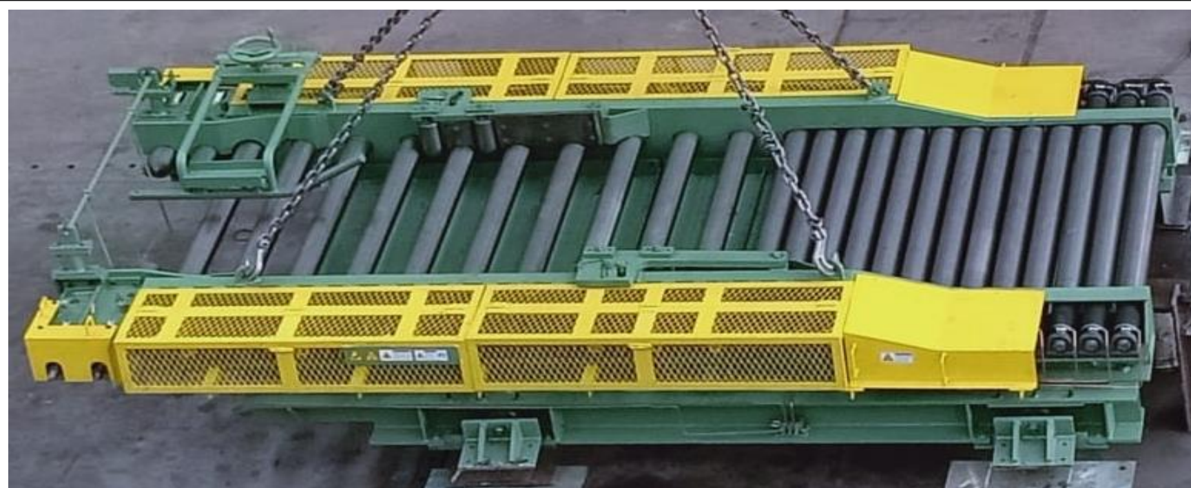
Roller Table for Stelmor Conveyor
